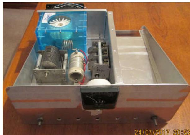
All of the metal and plastic work is home made so things proceed slowly. The space on the right is for the VHF amplifier which uses physically smaller fixed and variable components and has its own fan which has yet to be fitted. The tuning control positions on the front panel have yet to be determined, hence the remaining masking tape. Some form of flexible couplings will connect the front panel controls to the variable component shafts.
