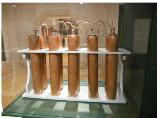
show 8 such cells connected together in series to form a 'battery', with each cell generating about 1.1 Volts.
